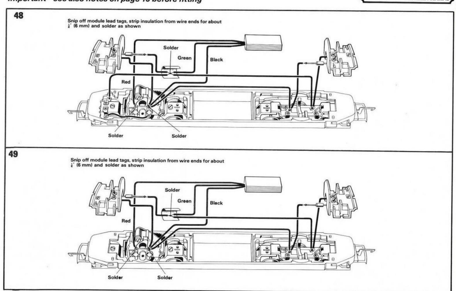
Module lead tag fitted onto existing light lead tag.
